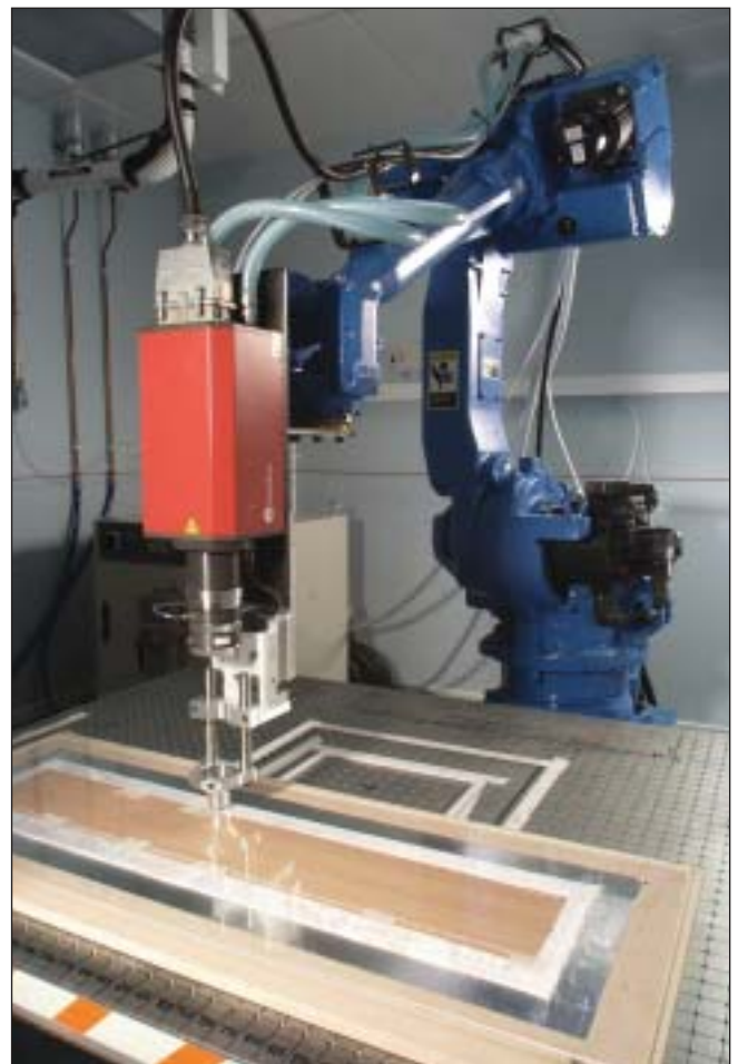
Robotic manipulation of diode laser welding upholstery to polyvinyl chloride-coated wooden divan drawer.
